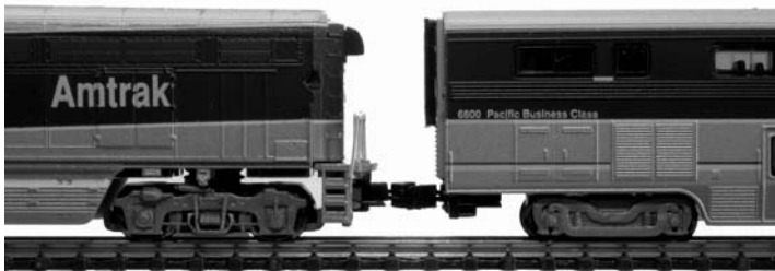
The clip alignment has been corrected and the DCC pocket has been filed down. The couplers now align correctly.
