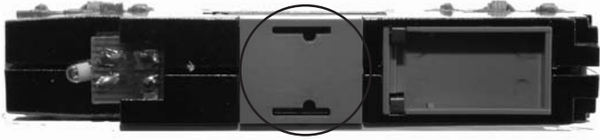
Figure 2: The holes in the top gray clip. These should be aligned towards the rear of the chassis as shown.
